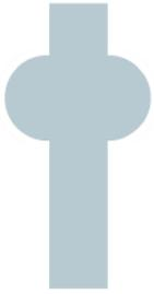
A Solid PTFE Type I gasket is guaranteed to fail in SIP conditions. They will creep, cold flow and leak at  $\Delta T$ .
